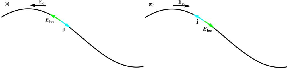
FIG. 3. (a,b) Sketch of a cross-section of a bump on a wire surface by a plane that is parallel to a wire axis. A projection of a constant electric field  $E_0$  onto a surface,  $E_{loc}$ , drives the electromigration adatom flux  $j$  in the opposite direction, i.e. in the direction of the electron flow  $j_e$ . This contributes to either (a) a bump smoothing (stabilization), or to (b) a bump growth (destabilization).
