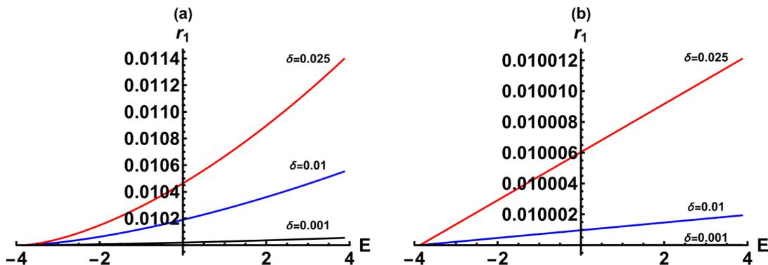
FIG. 6. The amplitude of  $\cos ky$  term in the ansatz (22), given by Eq. (29), at  $t_0 = 1$ ,  $\xi_0 = 0.01$  for  $E_c + 0.01 \leq E \leq -E_c$ , where  $E_c = -3.866$ . (a) Near the short-wave instability cut-off; (b) Near the long-wave instability threshold.
