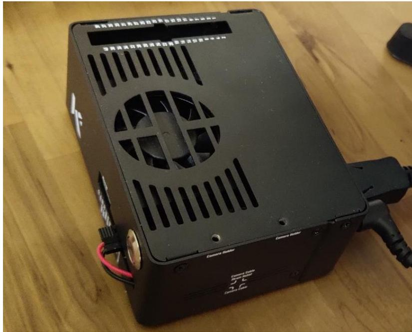
**Figure 3:** The NVIDIA Jetson Orin Nano board is housed inside a stainless-steel case. At the back are the power inlet, ethernet port, HDMI port and USB slots. The maximum power is 15 W, and the board is cooled by a fan assembly.
