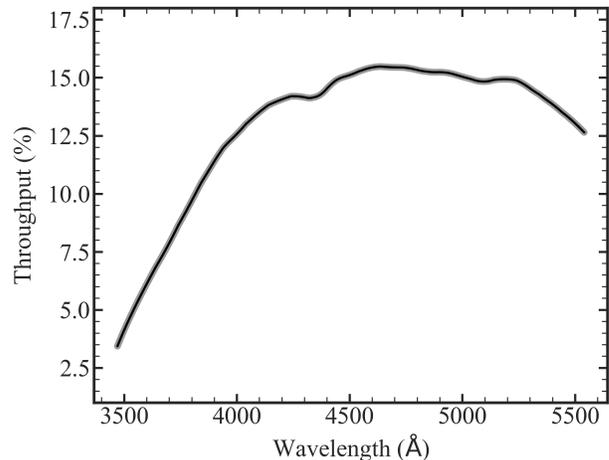
**Figure 3.** The Remedy VIRUS throughput curve used for the HETVIPS flux calibration. The curve is quite similar to that of Figure 17 in Hill et al. (2021) despite a different derivation and this work's throughput curve is plotted for an effective mirror illumination of  $50 \text{ m}^2$  rather than a full  $10\text{-m}$  aperture.
