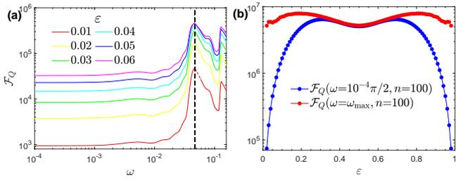
FIG. 3: (a) The QFI versus  $\omega$  in a chain of size  $L=20$  after  $n=10$  period cycles for different  $\varepsilon$ . The dashed line determines the onset of the phase transition. (b) The QFI versus  $\varepsilon$  for two values of  $\omega$ , obtained after  $n=100$  cycling periods in a system of size  $L=12$ .
