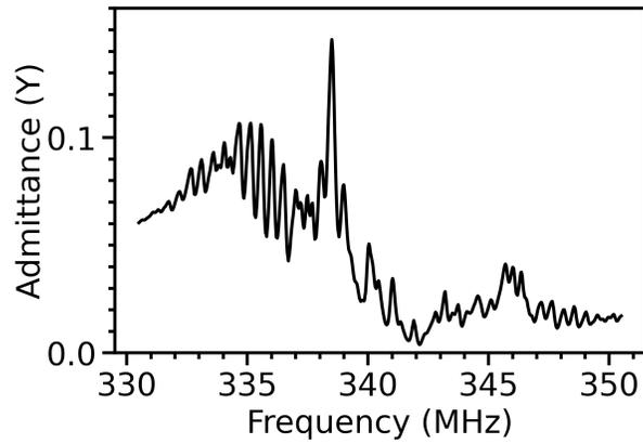
**Figure S1: Electrical verification of the SAW resonance.** The admittance  $Y$  parameter measured using an Agilent N5230A vector network analyzer, prior to mounting the device for the s-FFDXM experiment. The result shows an anti-resonance frequency at around 342 MHz, a resonance frequency at around 339 MHz.
