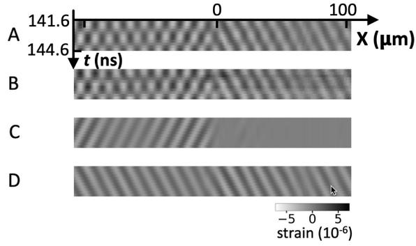
**Figure S6: Spatiotemporal strain map of the parasitic excitation.** (A) Summed contributions from  $\psi_{x+}$  and  $\psi_{x-}$  in the region near  $Z = 30 \mu\text{m}$  from  $t = 141.6$  to  $144.6$  ns. (B) Experimental spatiotemporal strain map previously shown in Figure 3C. The colormap is rescaled to improve the visibility of the weak wave amplitudes. Spatiotemporal strain map for individual wave components is shown for (C)  $\psi_{x-}$  and (D)  $\psi_{x+}$ .
