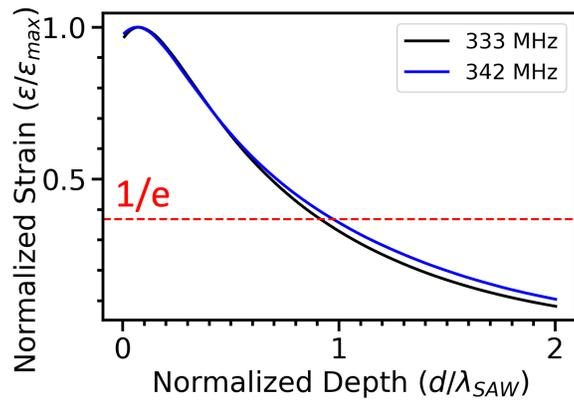
**Figure S9: FEM calculated SAW amplitude as a function of depth.** The SAW amplitude is normalized to its maximum value while the penetration depth is normalized by the device period  $\lambda_{SAW}$ . It can be seen that the SAW amplitude drops to  $1/e$  of its maximum value at around the depth of one  $\lambda_{SAW}$  for both 333 and 342 MHz.
