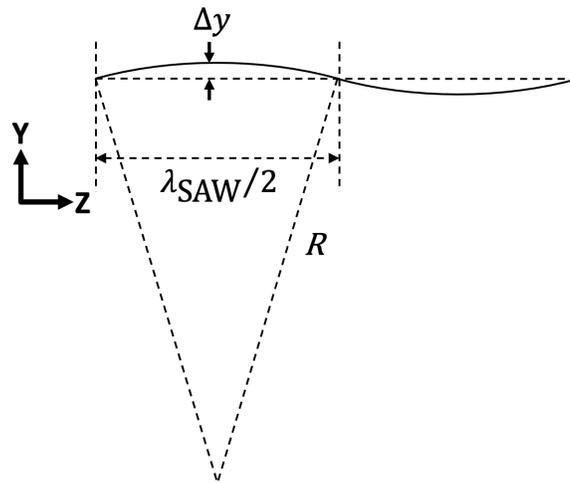
**Figure S11: Schematic for calculating the radius of curvature at the surface.** The SAW travels in the  $Z$  direction at a period of  $\lambda_{\text{SAW}}$ , causing surface displacement in the  $Y$  direction.
