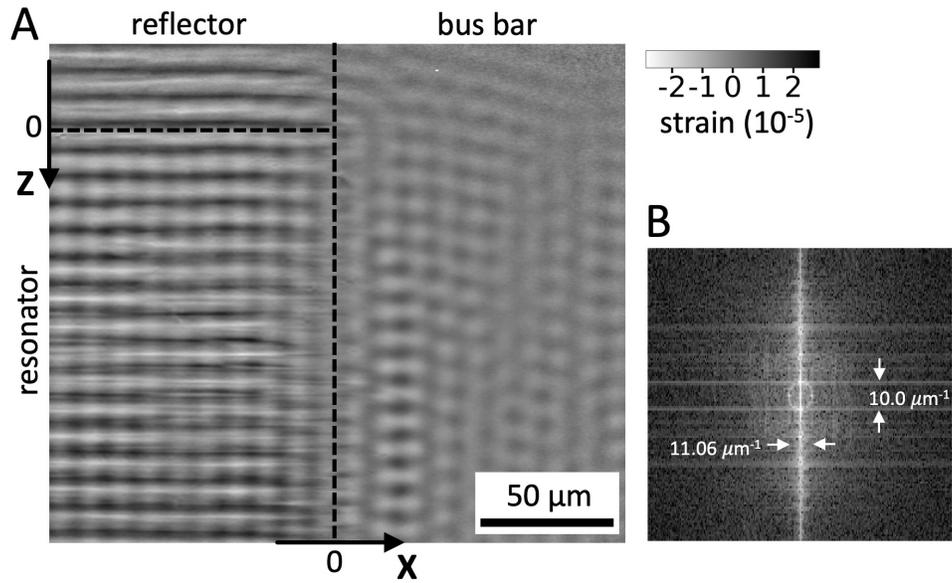
**Figure S2: Evidence of the two-dimensional wave pattern.** (A) Strain map of the SAW device at  $t = 143.1$  ns for an excitation frequency of 333 MHz. (B) FFT result on the resonator area for the strain map shown in (A).
