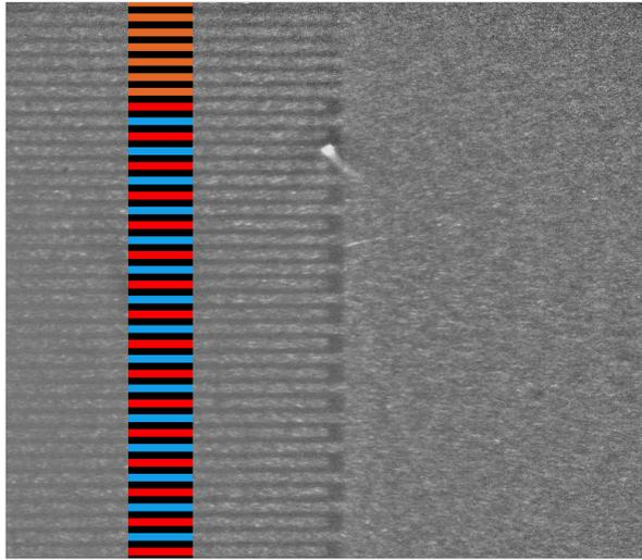
**Figure S3: Position of the IDT electrodes and reflector gratings.** FFDXM image taken without electrical excitation at  $\Delta\theta = -0.2^\circ$  off the Bragg peak. At this angle, the metallization layers are visible as they introduces weak contact strain on the  $\text{LiNbO}_3$  substrate. The  $Z$  positions of the electrode are then extracted and used to identify the reflector area, as well as the nodes and anti-nodes in the resonator area.
