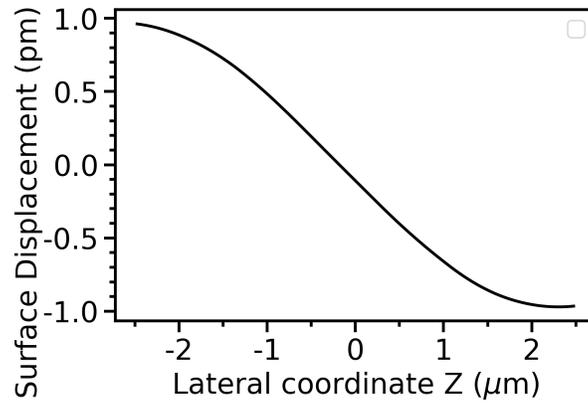
**Figure S10: FEM calculated surface displacement at 333 MHz.** For a strain of  $10^{-7}$ , the magnitude of the maximum displacement is about 1 pm.
