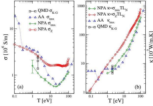
FIG. 4. (Color online) (a) The isochoric conductivities  $\sigma_z, \sigma_{tmx}$  calculated via the Ziman formula with NPA inputs, for  $l$ -aluminum, compared with selected AA and all QMD results as reported in Ref. [2]. (b) The NPA- $\kappa$  obtained via Eq.11, as well as selected thermal conductivities  $\kappa$  reported in Ref. [2].
