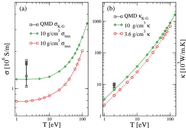
FIG. 2. (Color online) (a) The isochoric conductivities  $\sigma_{tmx}$  for  $l$ -carbon at  $10 \text{ g/cm}^3$  and  $3.6 \text{ g/cm}^3$  from NPA calculations. (b) The corresponding NPA- $\kappa$  obtained via the Lorentz number  $L_N(t)$ . The QMD results for  $\sigma$  and  $\kappa$  for  $l$ -C at  $10 \text{ g/cm}^3$ ,  $T=2 \text{ eV}$  reported in Ref. [17] are also displayed.
