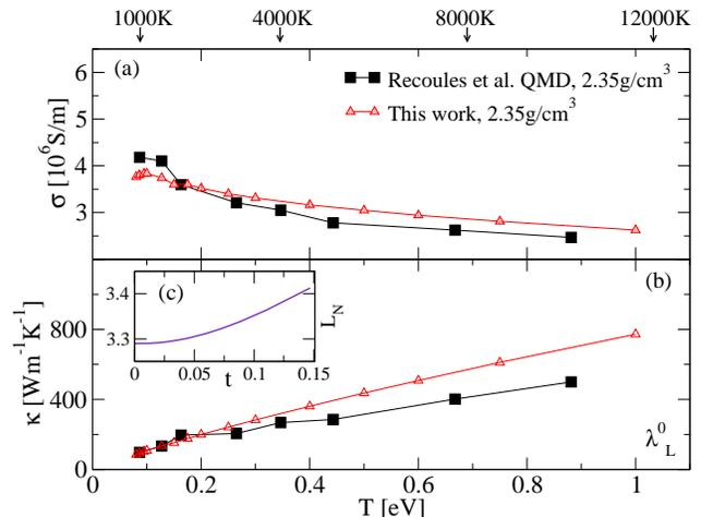
FIG. 2. (Color online) (a) The electrical conductivity  $\sigma_z$  for  $l$ -Al at  $2.35 \text{ g/cm}^3$  from the NPA-pseudopotentials and the Ziman formula. The QMD-KG results of Recoules et al [23] are at  $2.35 \text{ g/cm}^3$ . Panel (b) shows the corresponding  $\kappa$ . The inset (c) shows  $L_N(t), t = T/E_F$  Eq. 11 used in calculating  $\kappa$ .
