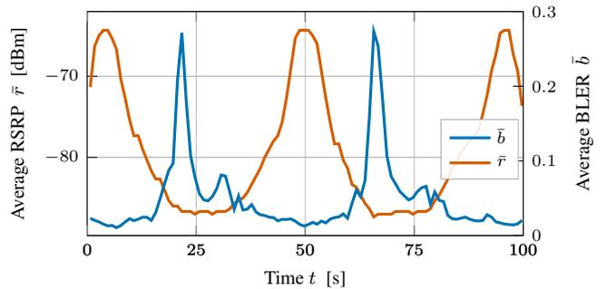
Figure 3: State of the wireless channel between the three vehicles and the gNB.
