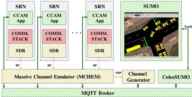
Figure 1: ColosSUMO architecture. Vehicular components are shown in green, while the wireless communication components are in yellow.
