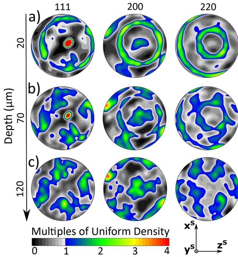
Figure 3: Comparisons of the measured textures in the NF (no finish) specimen at various depths: a) 20  $\mu\text{m}$ , b) 70  $\mu\text{m}$ , and c) 120  $\mu\text{m}$ .
