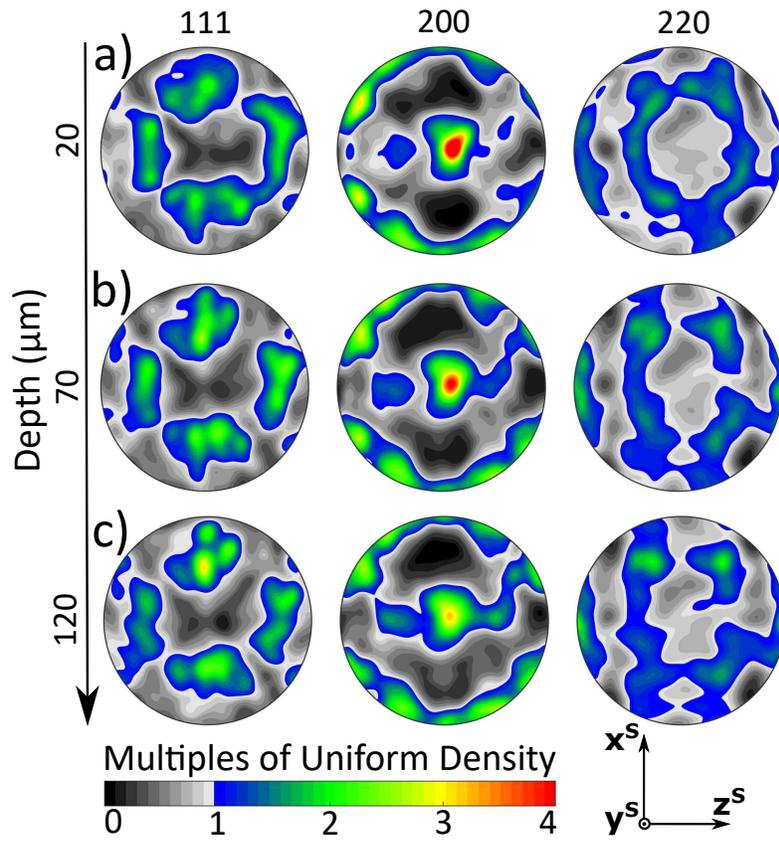
Figure 4: Comparisons of the measured textures in the U1 ( $6 \times 6$  SCT media, 75 mins) surface-finished specimen at various depths: a) 20  $\mu\text{m}$ , b) 70  $\mu\text{m}$ , and c) 120  $\mu\text{m}$ .
