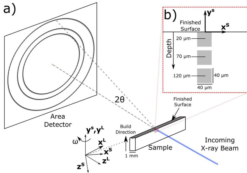
Figure 1: a) Experimental geometry for the X-ray diffraction measurements. The sample (S) and laboratory (L) coordinate systems are denoted. The sample is rotated by angle  $\omega$  to probe various sample directions and measured diffracted intensity positions are quantified by the exit angle  $2\theta$ . b) Inset showing the positions of diffraction volumes with respect to the finished surface in the probed specimens.
