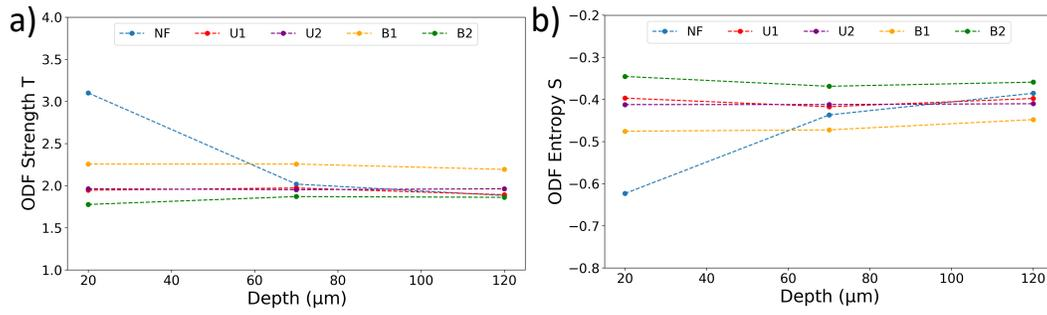
Figure 6: a) Variation of the ODF strength  $T$  in the five specimens as a function of depth. b) Variation of the ODF strength  $S$  as a function of depth.
