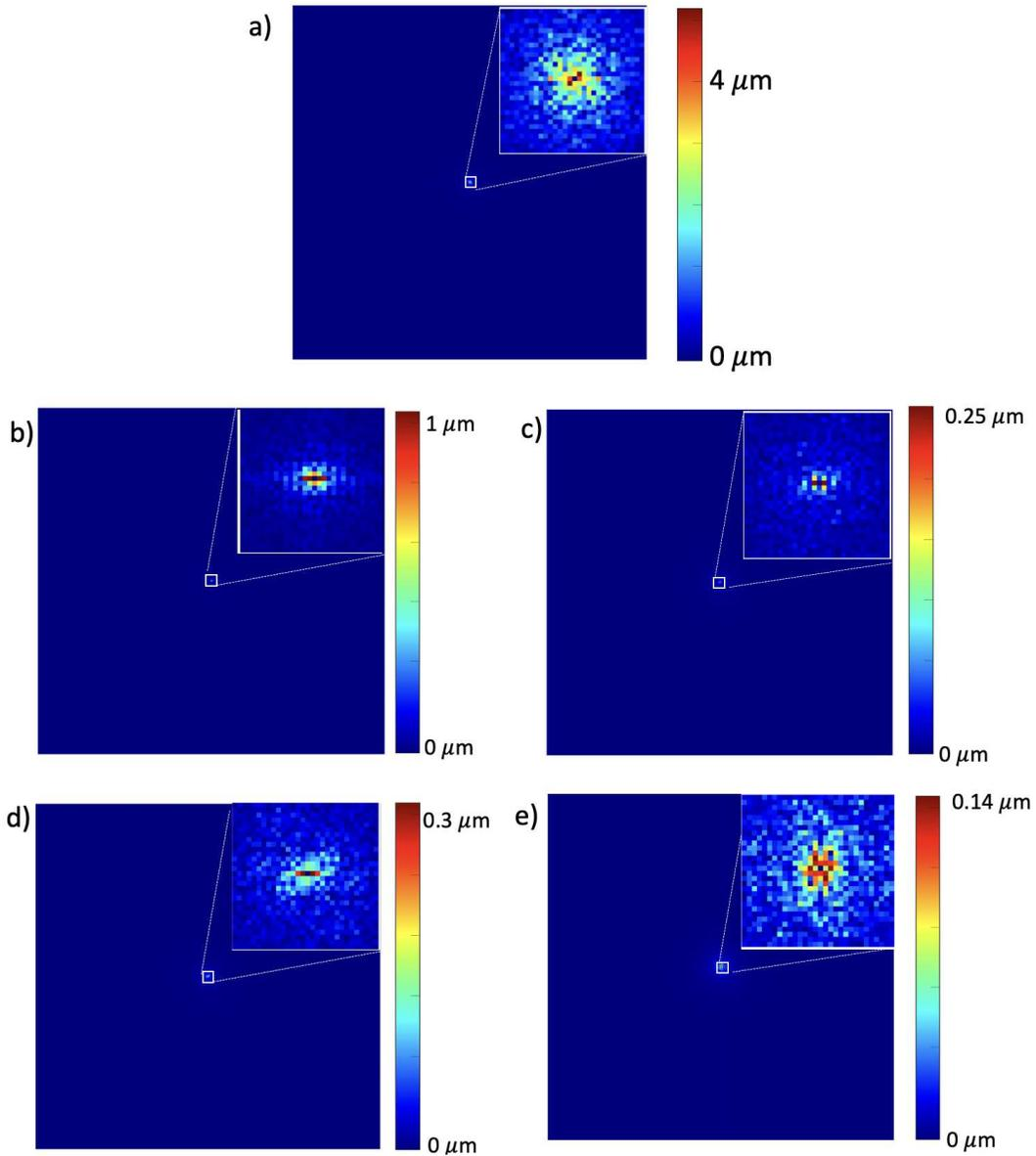
Figure 9: Fourier series analysis of surface topographies of representative specimens in various stages of CDF. a) NF (not finished), b) U1 (6x6 SCT media, 75 mins), c) U2 (6x6 SCT media, 135 mins), d) B1 (bimodal media, 75 mins), e) B2 (bimodal media, 135 mins). Spectrums are center-shifted and correspond to the original surface textures shown in Fig. 2. The insets show closeups of the central portions of these spectrums. Dimensions of the insets are 31x31 wavenumbers.
