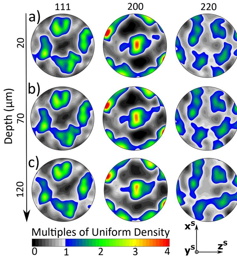
Figure 5: Comparisons of the measured textures in the B1 (bimodal media, 75 mins) surface-finished specimen at various depths: a) 20 μm, b) 70 μm, and c) 120 μm.
