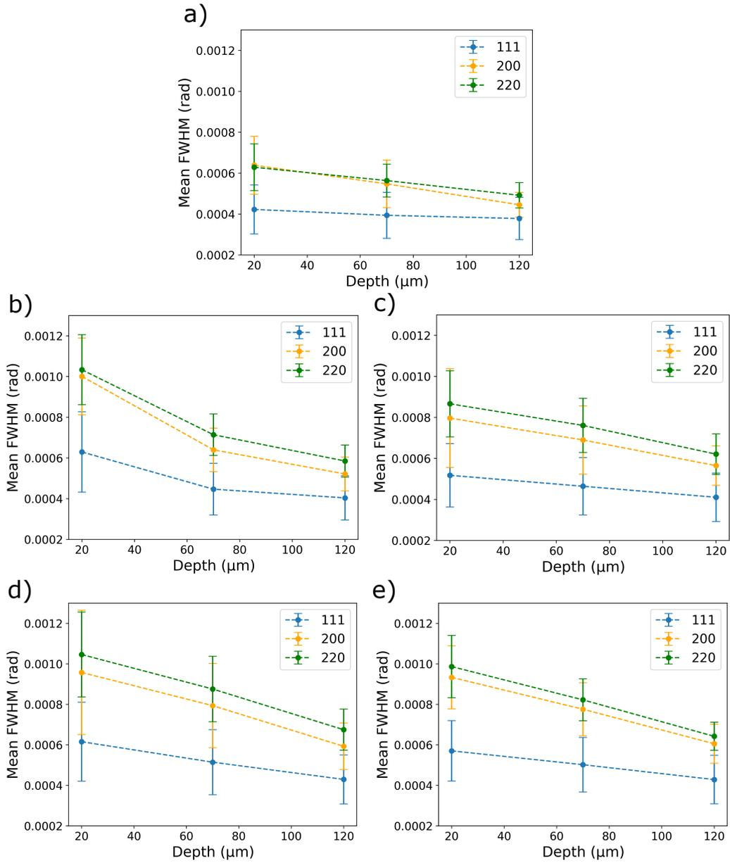
Figure 8: Comparison of the mean (data points) and standard deviation (error bars) of anisotropic diffraction peak FWHM with depth below the finished surface. Data from the 111, 200, and 220 diffraction peaks are shown. Data is presented from the a) NF (not finished), b) U1 (6 $\times$  6 SCT media, 75 mins), c) U2 (6 $\times$  6 SCT media, 135 mins), d) B1 (bimodal media, 75 mins), e) B2 (bimodal media, 135 mins) specimens.
