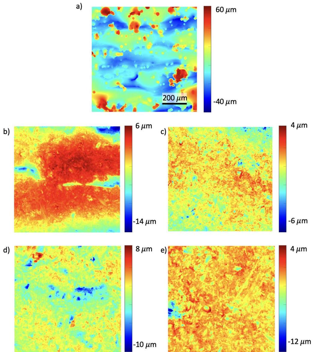
Figure 2: Surface topographies of representative specimens in the following stages of CDF: a) NF (not finished), b) U1 (6x6 SCT media, 75 mins), c) U2 (6x6 SCT media, 135 mins), d) B1 (bimodal media, 75 mins), e) (bimodal media, 135 mins).
