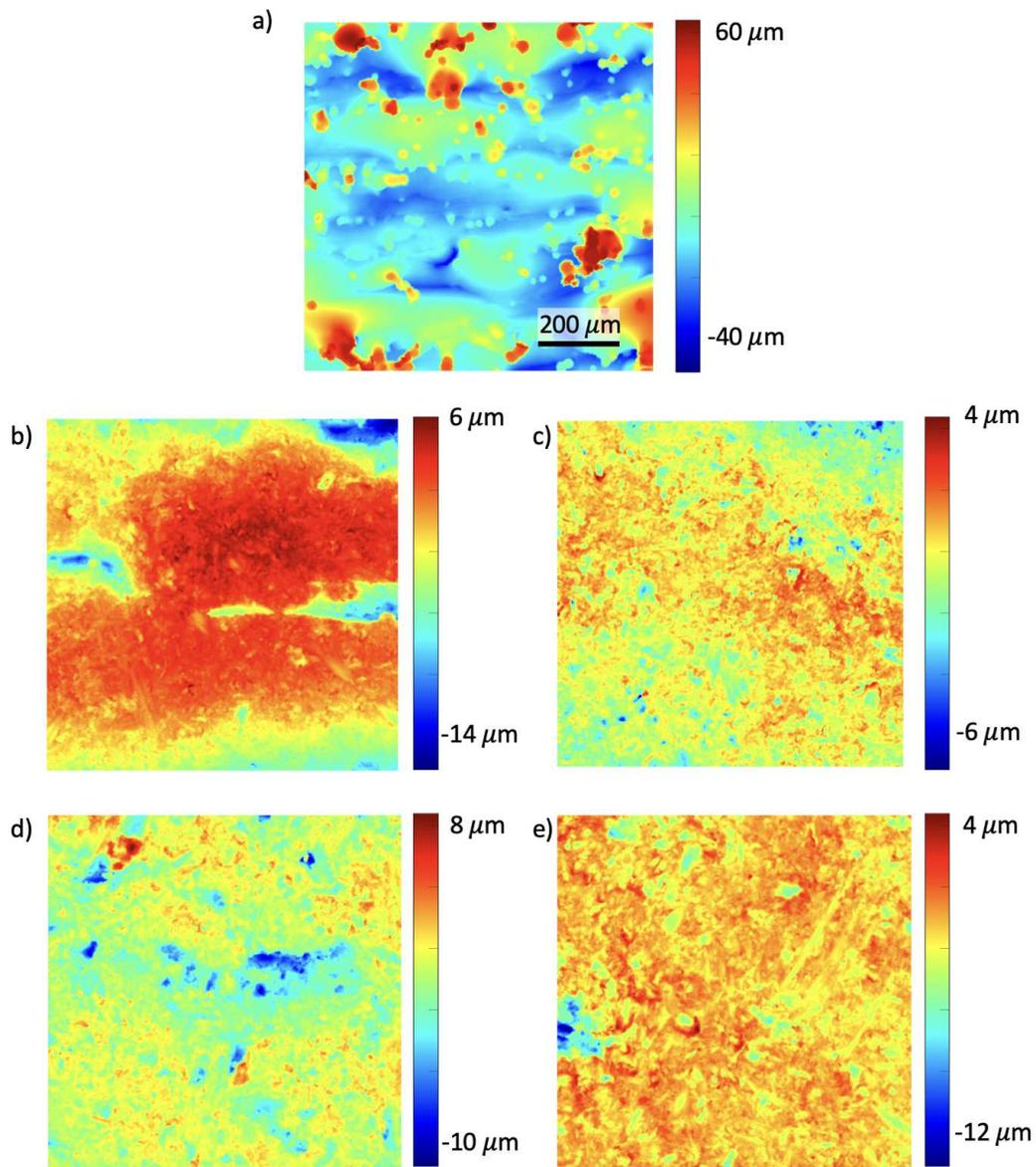
Figure 2: Surface topographies of representative specimens in the following stages of CDF: a) NF (not finished), b) U1 (6× 6 SCT media, 75 mins), c) U2 (6× 6 SCT media, 135 mins), d) B1 (bimodal media, 75 mins), e) (bimodal media, 135 mins).
