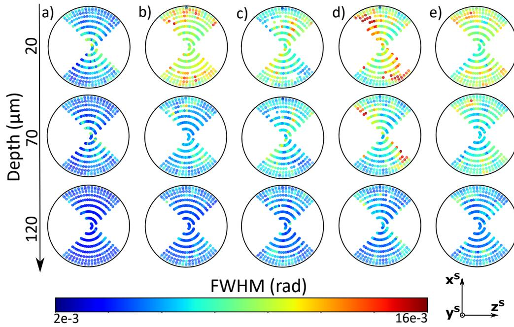
Figure 7: Comparison of 200 diffraction peak FWHM as a function of sample direction and depth below the finished surface. Data is presented from the a) NF (not finished), b) U1 (6x6 SCT media, 75 mins), c) U2 (6x6 SCT media, 135 mins), d) B1 (bimodal media, 75 mins), e) B2 (bimodal media, 135 mins) specimens.
