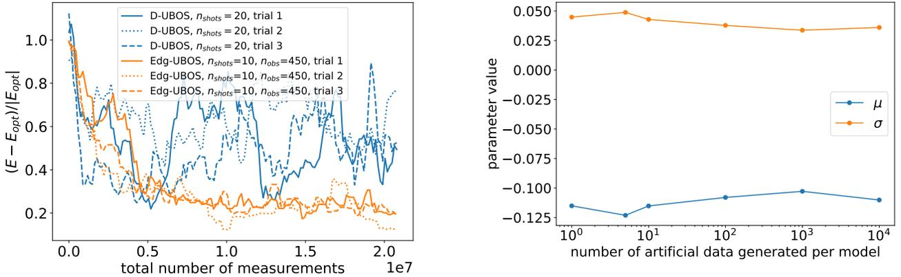
FIG. A4: Relative energy error for  $n_q = 8$  and  $n_d = 4$  as a function of total number of measurements during three different optimization runs of D-UBOS (blue; 20 shots per circuit) and Edg-UBOS (orange; 10 shots per circuit, 450 observations, which correspond to the same number of measurements per UBOS step).
