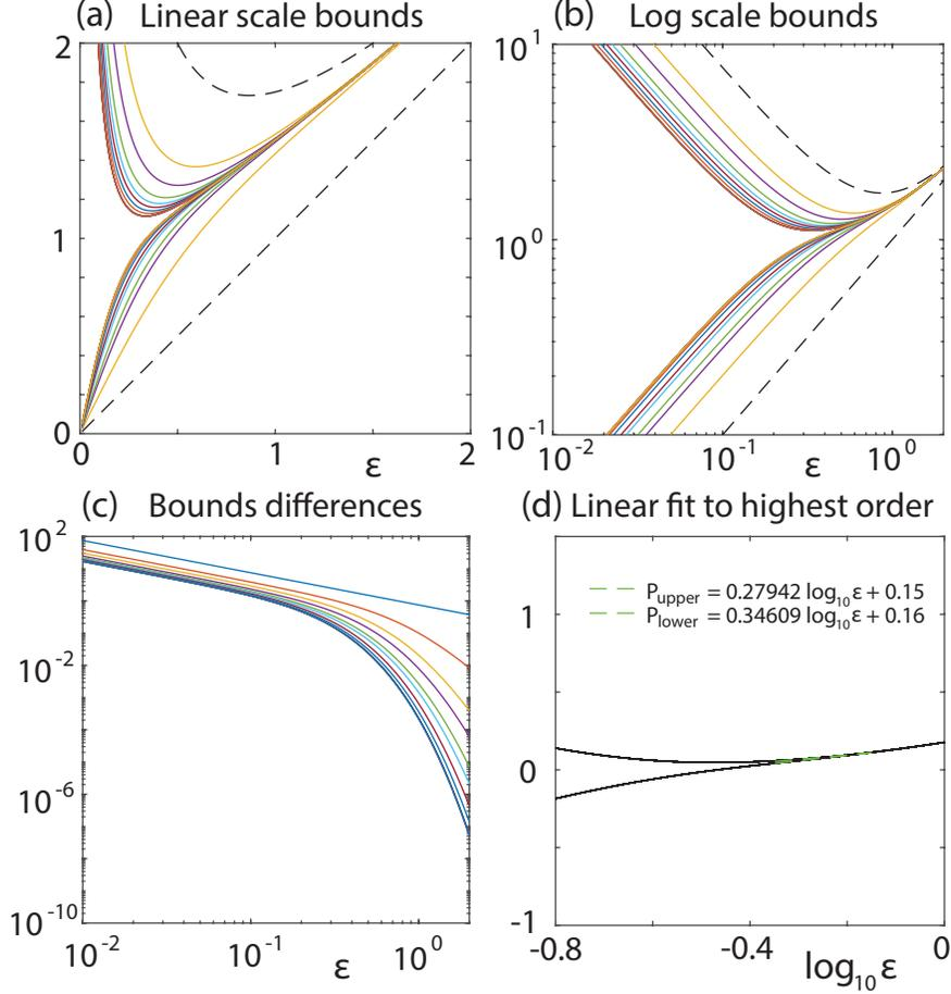
Figure 6: **Effective diffusivity bounds for space-time periodic flow.** Padé approximant upper  $[N/N]$  and lower  $[N - 1/N]$  bounds for  $N = 1, \dots, 8$  in linear scale (a) with corresponding absolute differences (b), and upper and lower bounds in log-log scale (c) in the variable  $\varepsilon$ . (d) Linear polynomial fits to the highest order upper and lower bounds with  $N = 8$ .
