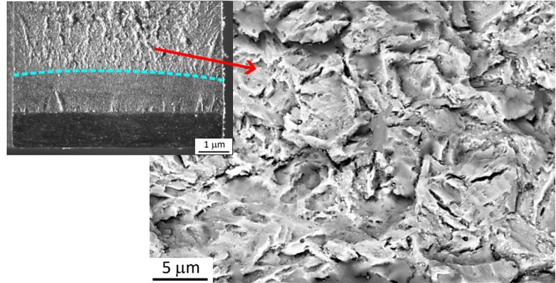
Fig. 12. Representative images for the fracture surfaces of specimens that (a) passed the 720-hour SENT test and were fractured in air and (b) failed the SENT test, exhibiting hydrogen-assisted quasi-cleavage fracture morphology. The dashed blue lines delimit the end of the fatigue pre-crack.
