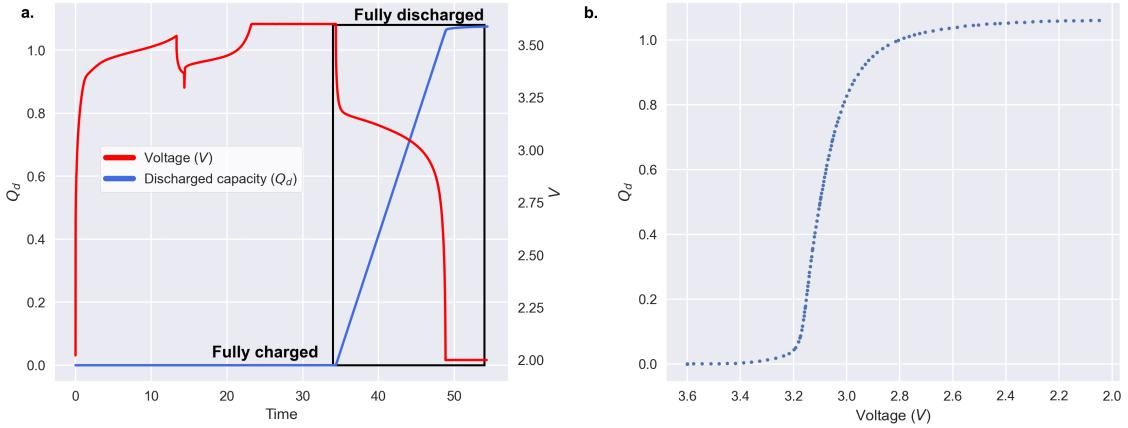
Figure 1: (a) Discharged capacity,  $Q_d(t)$ , and voltage,  $V(t)$ , measured for one battery over the course of a charge-discharge cycle. The discharge portion of the cycle is boxed in black. (b) The discharge-voltage curve,  $Q_d(V)$ , for the same battery. N.B.: the x-axis in (b) is flipped to reflect voltage decreasing over the course of the discharging process.
