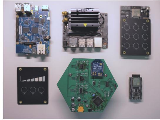
Fig. 14. Misaka core and its compatible extensions
