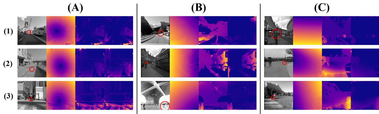
Figure 5: Visualization of ego-motion compensation, each image consists of four cells, from left to right: grayscale image with predicted moving direction, the magnitude of camera noise  $\epsilon$  (ego-motion), raw optical flow, and optical flow with ego-motion compensation.
