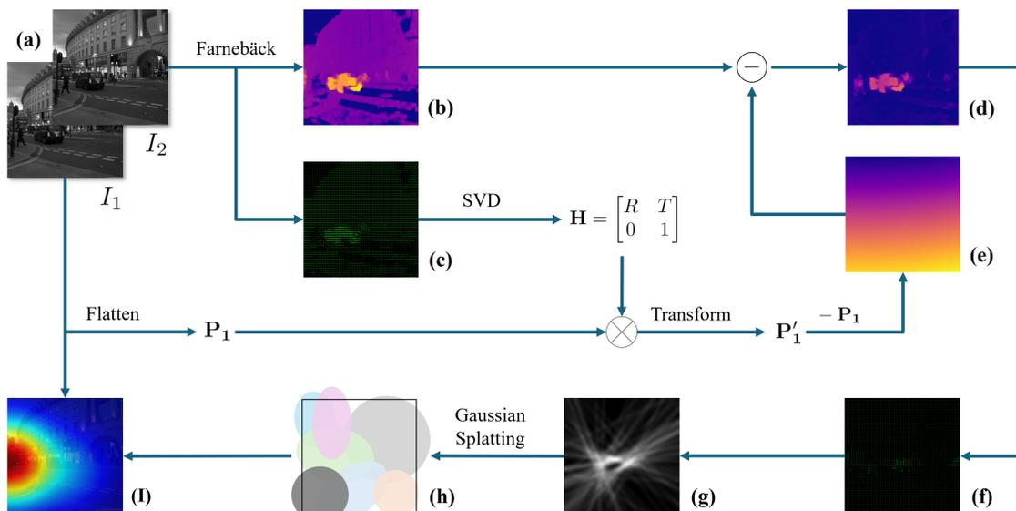
Figure 2: Framework, (a) is a two consecutive frame pair, (b) is the original optical flow, (c) is the original optical flow field, (d) is the compensated optical flow field, (e) is the camera noise  $\epsilon$ , (f) is the compensated optical flow field, (g) is the probability map of motor focus for  $I_2$ , (h) is the aggregated gaussian distribution of consecutive frames, and (i) is the attention map for motor focus of frame  $I_2$ .
