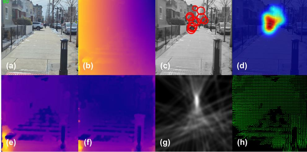
Figure 3: Motor focus visualization, (a) is the raw RGB image, (b) is the camera noise  $\epsilon$ , (c) is the attention area of 10 consecutive frames, (d) is the attention map aggregated by the gaussian distributions of 10 recent frames, (e) is the original optical flow, (f) is the compensated optical flow, (g) is the probability map of focus center, and (h) is the compensated optical flow field.
