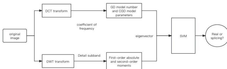
Figure 4: Flowchart of the stitching algorithm
