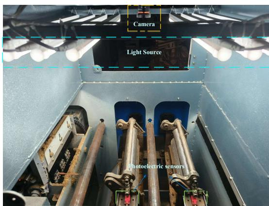
(a) inside wood plate image acquisition device
