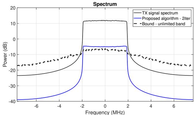
Fig. 4: Spectrum for the TX signal and PAPR reduction signals (realistic and unlimited band bound).
