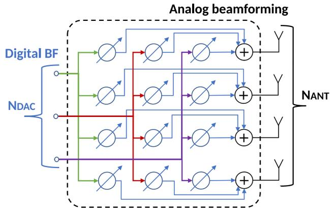
Fig. 1: Fully-connected HBF.
