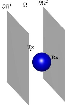
Fig. 3. MCvD system between two infinite reflecting surfaces.
