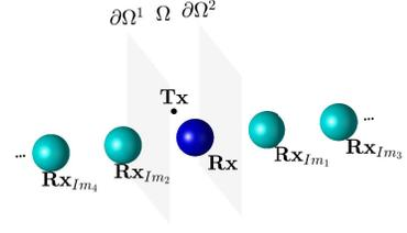
Fig. 4. Approximated SIMO system when the two infinite reflecting surfaces are omitted.
