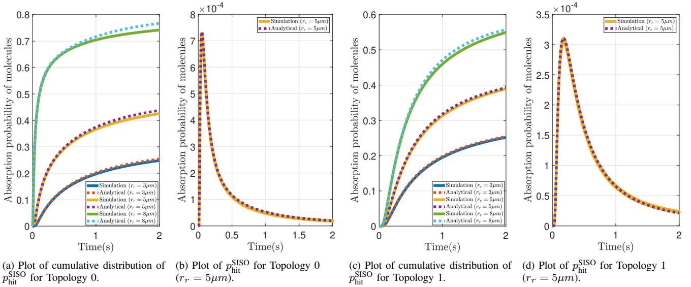
Fig. 6. Plots of absorption probabilities of molecules by Rx with radii  $3\mu\text{m}$ ,  $5\mu\text{m}$ , and  $8\mu\text{m}$  for Topology 0 and Topology 1.TABLE II
