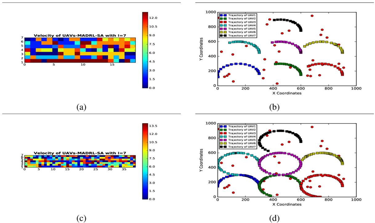
Figure 3.7: Velocities and trajectories of MADRL-SA with  $I=7$ . (a) and (b) velocity and trajectory given number of waypoints=20. (c) and (d) velocity and trajectory given number of waypoints=40
