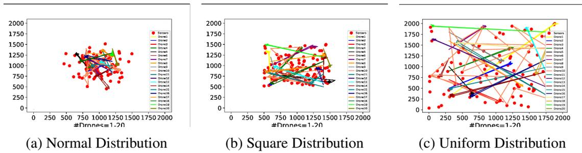
Figure 4.5: MF-HPPO trajectory distributions for various UAV counts and ground sensor distributions.
