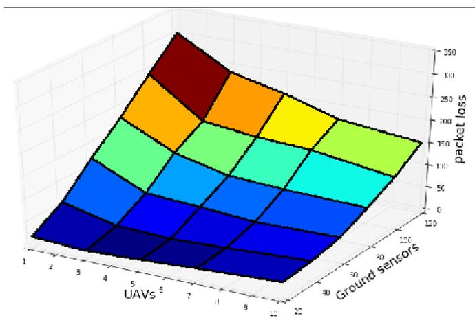
Figure 3.5: Trade-off between the number of UAVs and ground sensors.
