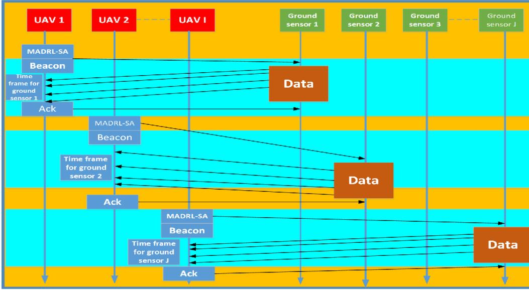
Figure 3.1: Data communication protocol for UASNets. MADRL-SA conducts velocity determination, sensor selection, and modulation scheme allocation in each communication frame
