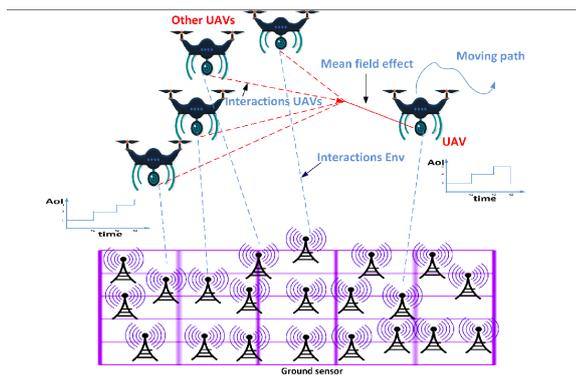
Figure 4.1: Mean field representation of UASNs.
