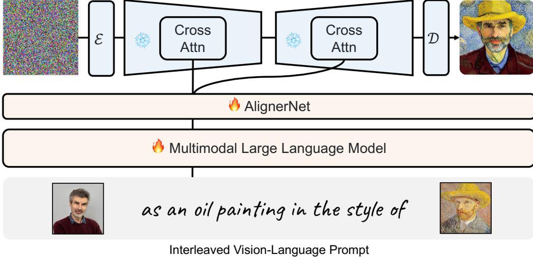
Figure 2: KOSMOS-G comprises an MLLM for multimodal perception, coupled with an AlignerNet that bridges the MLLM to the diffusion U-Net image decoder. KOSMOS-G can pass the fine concept-level guidance from interleaved input to image decoder, and offer a seamless alternative to CLIP. Orange denotes the trainable modules; Blue denotes the frozen ones.
