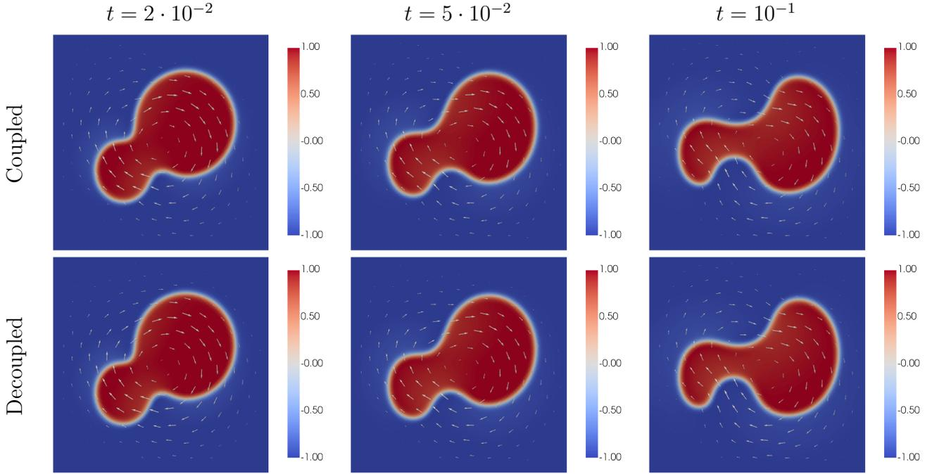
Figure 2: Evolution of  $\Pi^h \phi$  over time in Test 5.2 ( $\rho_1 = 1, \rho_2 = 100$ ).
