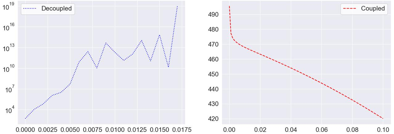
Figure 5: Left, discrete energy of the decoupled scheme. Right, discrete energy of the coupled scheme. Test 5.2 ( $\rho_1 = 1$ ,  $\rho_2 = 1000$ ).
