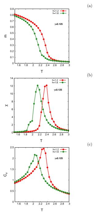
Figure 4: The (a) magnetization (m), (b) the susceptibility  $(\chi)$  and (c) the specific-heat  $(C_v)$  (c) are plotted against the temperature (T) for two different strengths of the uniform random fields, h = 1.2 and h = 1.6 with  $(\gamma = 0.125)$ .
