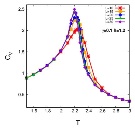
Figure 9: The specific heat  $(C_v)$  plotted as function of the temperature (T) for five different system sizes (L=10,15,20,25 and 30). Here, magnitude of the random field, h=1.2 and the strength of the anisotropy,  $\gamma=0.1$ . The random field (A-type) has the direction chosen randomly within angle 0 and  $2\pi$ .
