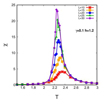
Figure 7: The susceptibility  $(\chi)$  plotted as function of the temperature (T) for five different system sizes (L=10,15,20,25 and 30). Here, magnitude of the random field, h=1.2 and the strength of the anisotropy,  $\gamma=0.1$ . The random field (A-type) has the direction chosen randomly within angle 0 and  $2\pi$ .
