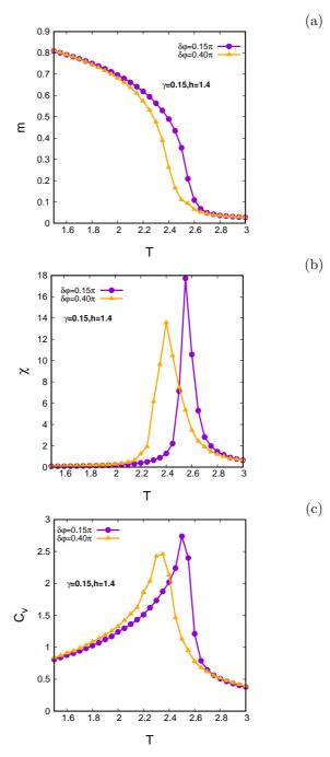
Figure 12: The (a) magnetization (m), (b) susceptibility  $(\chi)$  and (c) specific-heat  $(C_v)$  are plotted against temperature for two different angular window  $(\delta\phi=0.15\pi$  and  $\delta\phi=0.40\pi)$  with anisotropy  $\gamma=0.15$  and field strength h=1.4.
