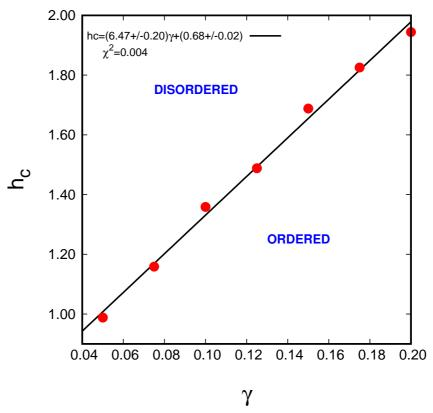
Figure 6: The compensating field  $(h_c)$  is plotted as function of the strength of anisotropy  $(\gamma)$ . The compensating field has been calculated from the linear interpolation around the true critical temperature  $(T_c = 2.206)[6, 7]$ . The data points are fitted with a straight line. The region of ordered and disordered phases are separated by this line.
