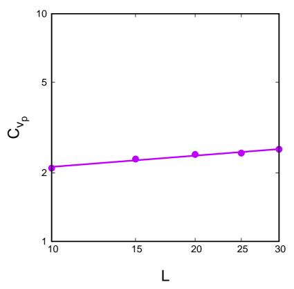
Figure 18: The logarithm of the heights of the peaks of the specific heat  $(C_{vp})$  are plotted against the logarithm of system sizes L, for h=1.4,  $\gamma=0.1$  and  $\delta\phi=0.3\pi$ . The data points are fitted with a straight line assuming the scaling law  $C_{vp}\sim L^{\alpha/\nu}$ . Here, we have estimated (from the linear best fit)  $\alpha/\nu=0.16\pm0.02$  having  $\chi^2=0.003$  and DOF=3. Here, the B-type random field is used.
