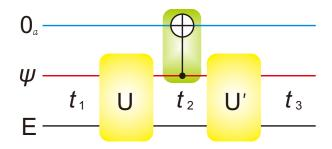
FIG. 1: Logic circuit to measure the value of  $K(t_2, t_3)$  with a CNOT gate.  $0_a$  is the initial state of the ancilla.  $\psi$  is the state of the system (can only be in 0 or 1 during the evolution under the classical realistic description). E represents the environment with operation of U between  $t_1$  and  $t_2$ , and U' between  $t_2$  and  $t_3$ , respectively.
