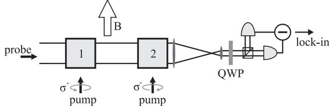
Fig. 3. Experimental setup. Cells 1 and 2 are placed in magnetic shields in equal magnetic fields  $\vec{B}$  oriented along  $x$ . The atoms inside are pumped with circularly polarized pump beams of opposite helicity. The probe beam propagates perpendicular to the  $\vec{B}$  field, interacts with the atoms and finally hits a balanced homodyne detector.
