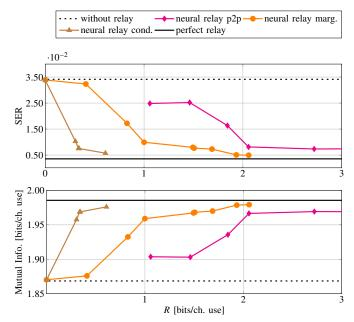
Fig. 3: Symbol error rate (SER) and mutual information as a function of the relay-to-destination rate R, for the 4-PAM modulation with  $\gamma_D = \gamma_R = 13$  dB. The colored lines represent the performance of three neural CF relay architectures (Fig. 2), where each marker corresponds to a unique model trained for a particular value of  $\lambda$  in (12). The horizontal black lines provide baseline results without relaying (R=0) and with perfect relaying  $(R\to\infty)$ .
