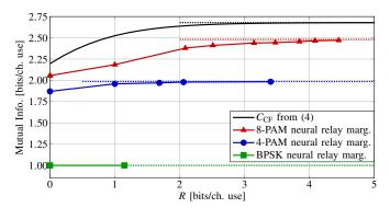
Fig. 6: Mutual information for the marginal model (Fig. 2a) in case of BPSK, 4-PAM and 8-PAM modulations with  $\gamma_D = \gamma_R = 13$  dB. The solid line represents  $C_{\rm CF}$  in (4) [15], obtained for Gaussian inputs. The dotted lines represent the perfect relay  $(R \to \infty)$  bounds for the respective curves, similar to Figs. 3, and 4.
