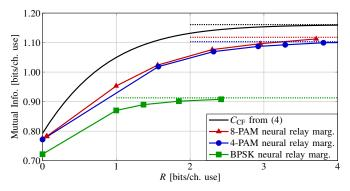
Fig. 5: Mutual information for the marginal model (Fig. 2a) in case of BPSK, 4-PAM and 8-PAM modulations with  $\gamma_D = \gamma_R = 3$  dB. The solid line represents  $C_{CF}$  in (4) [15], obtained for Gaussian inputs. The dotted lines represent the perfect relay  $(R \to \infty)$  bounds for the respective curves, similar to Figs. 3 and 4.
