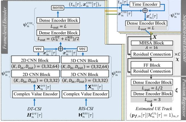
Fig. 3. Transformer-based tracking function  $f$  based on the hierarchical architecture proposed in the X<sup>2</sup>Track framework.
