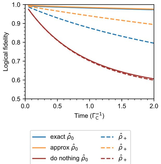
FIG. 5. Sequential correction of the logical states  $|\bar{0}\rangle$  (solid line) and  $|\bar{1}\rangle$  (dashed line) using the exact CS(7,2,5) (blue) and the approximate A(7,-2,2) (orange) error correction code for the correction rate  $\Omega_{\text{BSB}} = 500 \Gamma_C$ .
