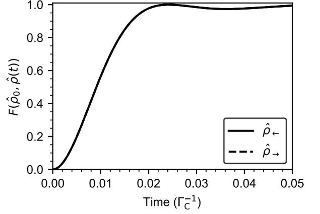
FIG. 9. Evolution of the physical fidelity  $F(\hat{\rho}_0, \hat{\rho}(t))$  after tracing out the motional modes for two different initial error states using the Zeeman DEC scheme.
