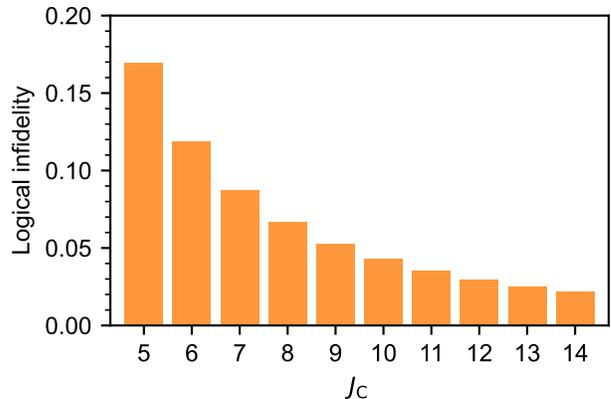
FIG. 3. Worst-case logical infidelity after a single error for the approximate  $A(J_C, -2, 2)$  quantum error correction code as a function of the code manifold  $J_C$ .
