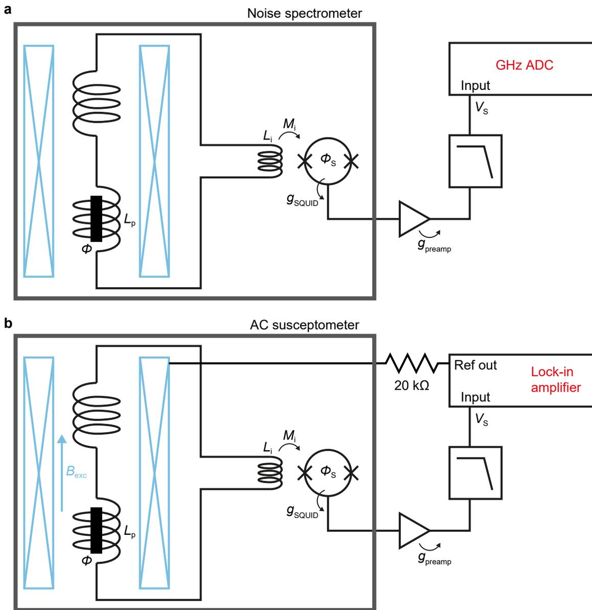
**Supplementary Fig. 5 Schematic circuit diagrams of the experiment.**
