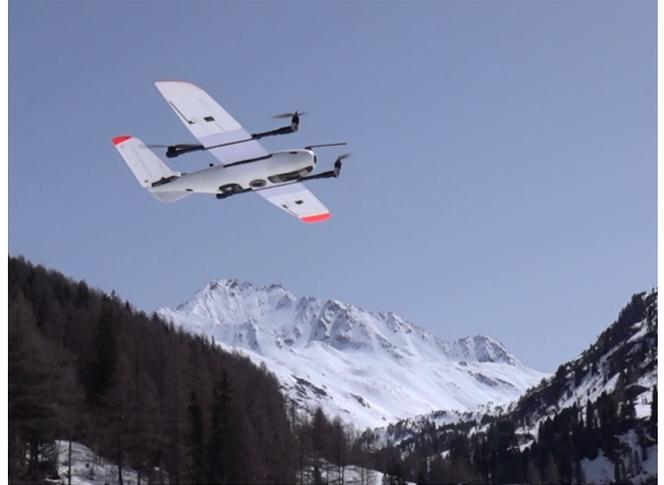
Fig. 1: Image of the tiltrotor VTOL platform during take-off during the field test in a narrow valley in Davos, Switzerland.
