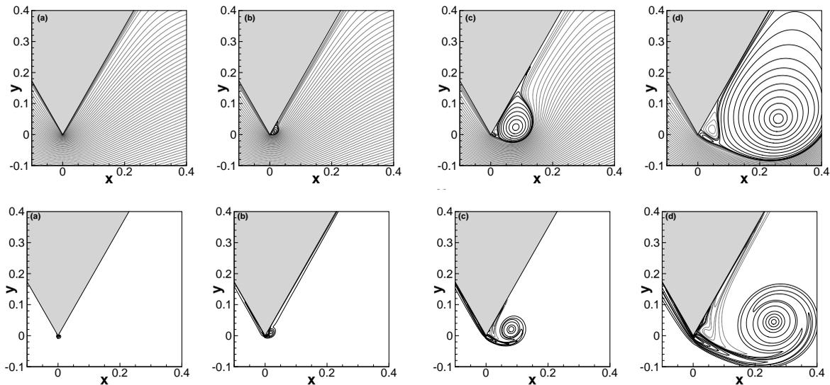
FIGURE 5. Four stages of flow evolution for  $Re_c = 1560$  at non-dimensional time (a)  $t = 0.001$ , (b)  $t = 0.01$ , (c)  $t = 0.10$  and (d)  $t = 0.40$ : Top row, the streamlines and Bottom row, the vorticity contours. The positive contours are in solid lines and negative contours are in dotted lines.
