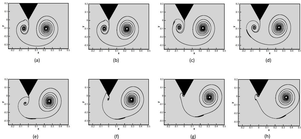
FIGURE 13. Streaklines at time  $t = 0.70$  for  $Re_c = 1560$  after the impulsive stop at time  $t = 0.435 + t_{dec}$  where  $t_{dec}$  is the length of the time interval over which the inlet velocity reduces to zero from a unit velocity. The deceleration starts at time  $t_f = 0.435$ . Top:  $t_{dec} =$  (a)0.002, (b)0.01, (c)0.03 and (d)0.05 (from left to right) and Bottom:  $t_{dec} =$  (e)0.10, (f)0.15, (g)0.20 and (h)0.25 (from left to right).
