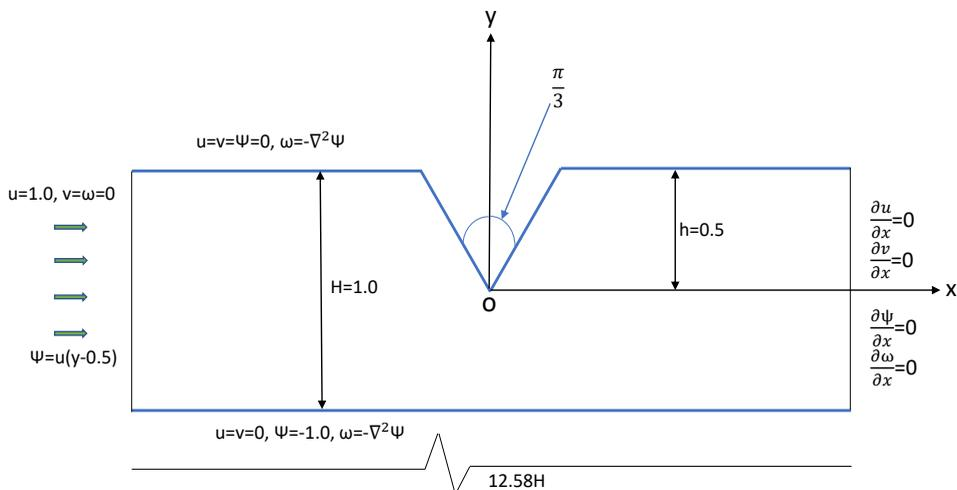
FIGURE 2. Problem statement of the flow past a mounted wedge in uniform flow.
