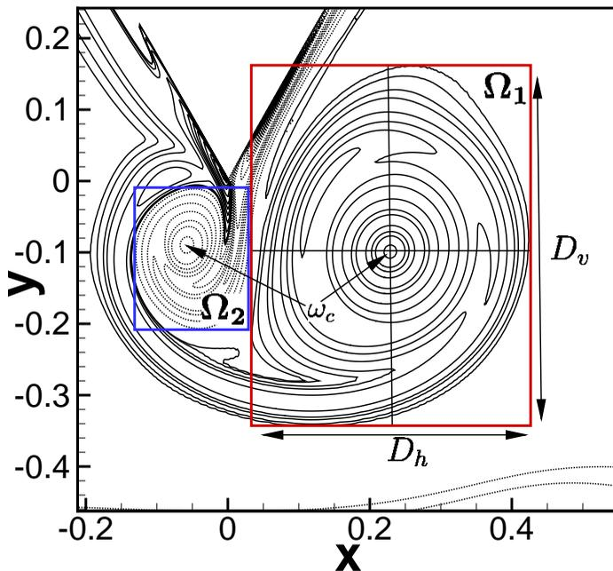
FIGURE 8. Schematic of vortex center, radius and circulation.
