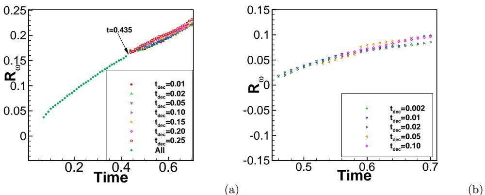
FIGURE 10. Evolution of radii  $R_\omega$  of the (a) starting and (b) the stopping vortices for different time intervals of deceleration.
