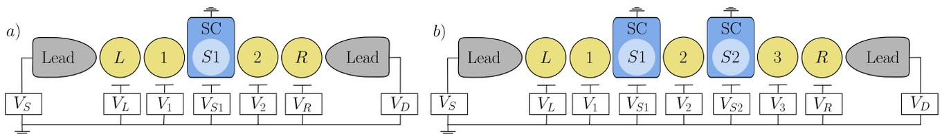
FIG. 1. Sketch of the artificial Kitaev chain systems considered in this paper. In addition to the sensor dots marked  $L/R$  on either side of the Kitaev chain, the array consists of (a) 3 dots or (b) 5 dots, where every other dot is proximitized by a superconductor (blue square) to create an Andreev bound state that can mediate CAR and ECT processes between the normal dots.
