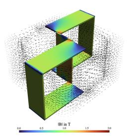
Fig. 2. Solution to the magnetostatic problem using our mixed approach. Black arrows depict the direction of the current in the coil. Scalar value is the magnitude of the b-field. (computed using Netgen/NGSolve and displayed using PyVista.
