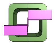
Fig. 1. Bird's eye view of the geometry of TEAM problem 13. Pink volumes are the steel plates; the green area is the coil. The ambient air box is hidden.
