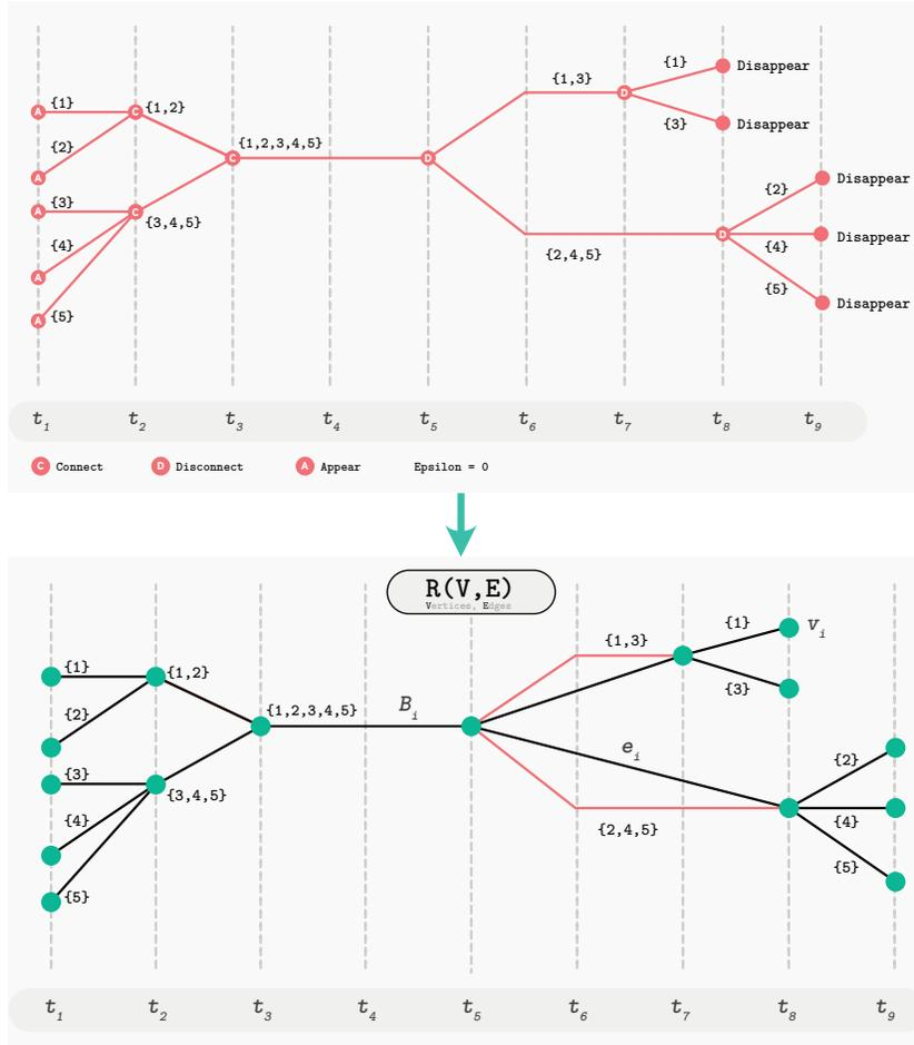
Fig. 2: REEB GRAPH CONSTRUCTION OVER TIME. We show the construction of Reeb graphs  $R(V, E)$  for a set of five trajectories. The *appear*, *disappear*, *connect*, and *disconnect* events are shown on the left-hand side. Changes in the grouping of trajectories due to these events are encoded as nodes on the right-hand side. Nodes of the Reeb graph  $\mathcal{R}$  on the right-hand side are shown in red color and the edges are shown in black color throughout the paper.
