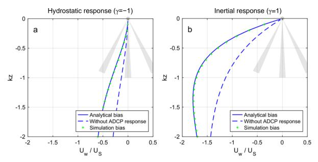
Fig. 11 Wave-induced tilt and motion biases in relative horizontal velocity measured by a downwardlooking ADCP mounted on a surface quasi-Lagrangian platform with a) hydrostatic and b) inertial responses. Analytical estimates with and without taking the ADCP beam response into consideration are shown in solid and dashed blue lines, respectively; the latter is the same as shown in Fig. 6 (blue line). Results of the semi-analytical simulation are shown for comparison (green dots).
