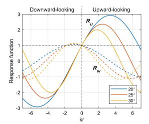
Fig. 8 ADCP response functions for horizontal ( $R_u$ , solid lines) and vertical ( $R_w$ , dashed lines) velocities as a function of normalized range (or wavenumber), kr. Response functions are shown for several typical ADCP beam angles. Positive values of kr correspond to upward-looking ADCPs.
