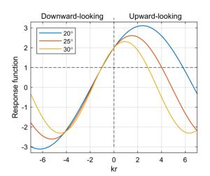
Fig. 10 ADCP response functions for "sweeping" horizontal velocity bias  $R_t$  as a function of normalized range (or wavenumber), kr. Response functions are shown for several typical ADCP beam angles. Positive values of kr correspond to upward-looking ADCPs.
