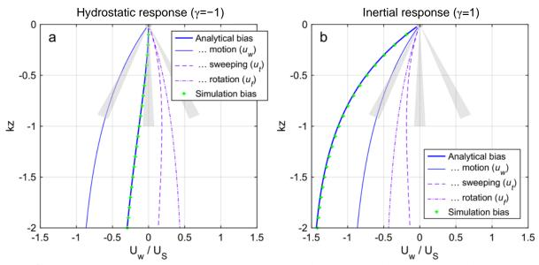
Fig. 6 Wave-induced tilt and motion biases in relative horizontal velocity measured by a surface downward-looking Lagrangian instrument with a) hydrostatic and b) inertial response. Estimates of motion bias  $(u_w, eq. (16))$ , sweeping tilt bias  $(u_t, eq. (27))$ , and frame rotation bias  $(u_f, eq. (31))$ , and total bias are shown. Results of the semi-analytical simulation are shown for comparison (green dots).
