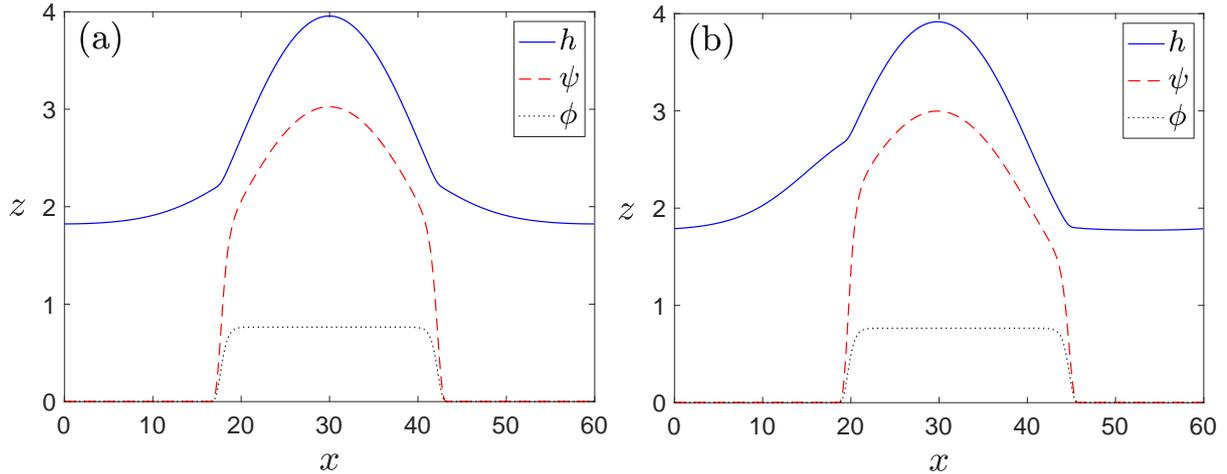
Figure 15: Profiles for a system of length  $L_x = 60$  and corresponding to the bifurcation diagrams in Fig. 14. Panel (a) shows the unstable symmetrical solution on the first colloid branch and (b) shows the stable asymmetrical solution on the side branch bifurcating from the first colloid branch.
