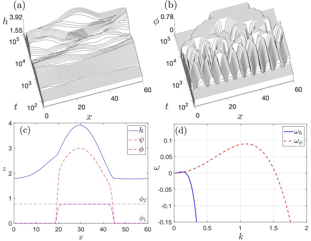
Figure 9: Panels (a) and (b) show waterfall plots over time (using  $\log t$ ) of the film height and the local colloid concentration, respectively, for  $A' = 1$ ,  $K' = 0.13$ ,  $\alpha' = \beta' = 3$ ,  $\epsilon' = 0.5$ ,  $a^2 = 2$ ,  $h_i = 2.5$  and  $\phi_i = 0.41$ . Panel (c) shows the final equilibrium profiles and (d) shows the dispersion relation for this system.
