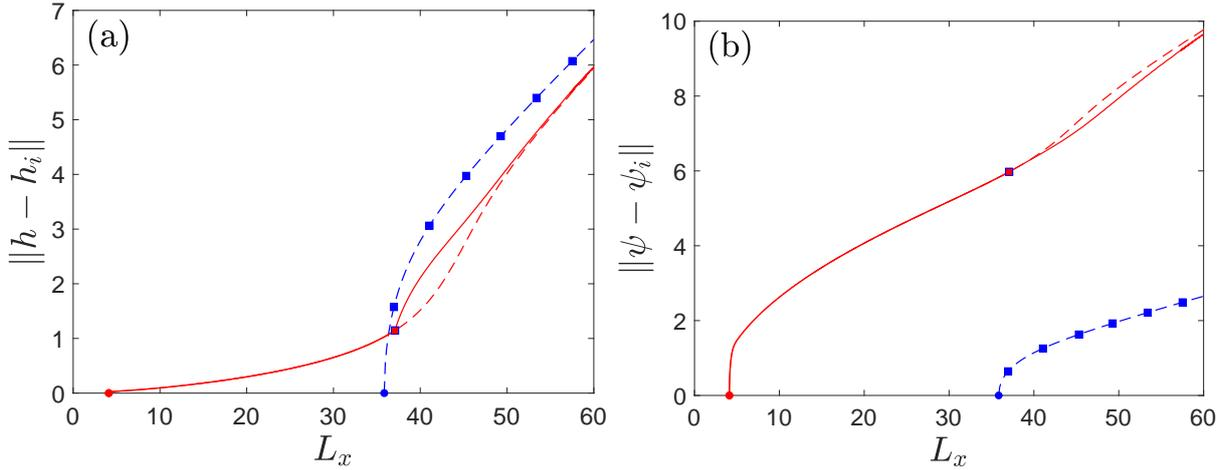
Figure 14: Bifurcation diagrams for the same parameters as in Fig. 9. Panel (a) shows the  $L^2$ -norm for  $h$ , while (b) shows this for  $\psi$ . The red dashed line is the solution branch corresponding to unstable equilibria with symmetrical profiles. The red solid line is for the stable equilibria, which to the right of the red square are asymmetrical. The blue dashed line corresponds to the unstable thin film branch of solutions.
