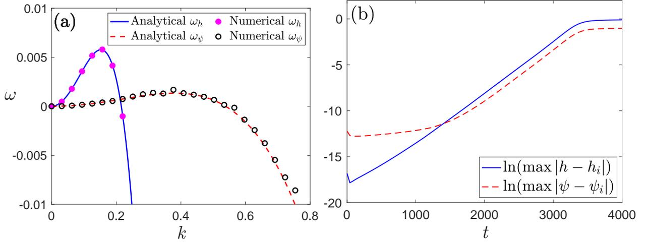
Figure 4: Results for a case with  $A' = 2$ ,  $K' = 0.15$ ,  $\alpha' = 1$ ,  $\epsilon' = 0.5$ ,  $a^2 = 2$ ,  $h_i = 2.2$ , and  $\phi_i = 0.4$ . (a) Dispersion relation calculated numerically via Eqs. (51) and (52) using  $\epsilon_h = 10^{-7}$ ,  $\epsilon_\psi = 10^{-5}$  (symbols) compared to the analytic results in Eqs. (33) and (34) (lines). (b) Measure of the evolution [c.f. Eq. (53)].
