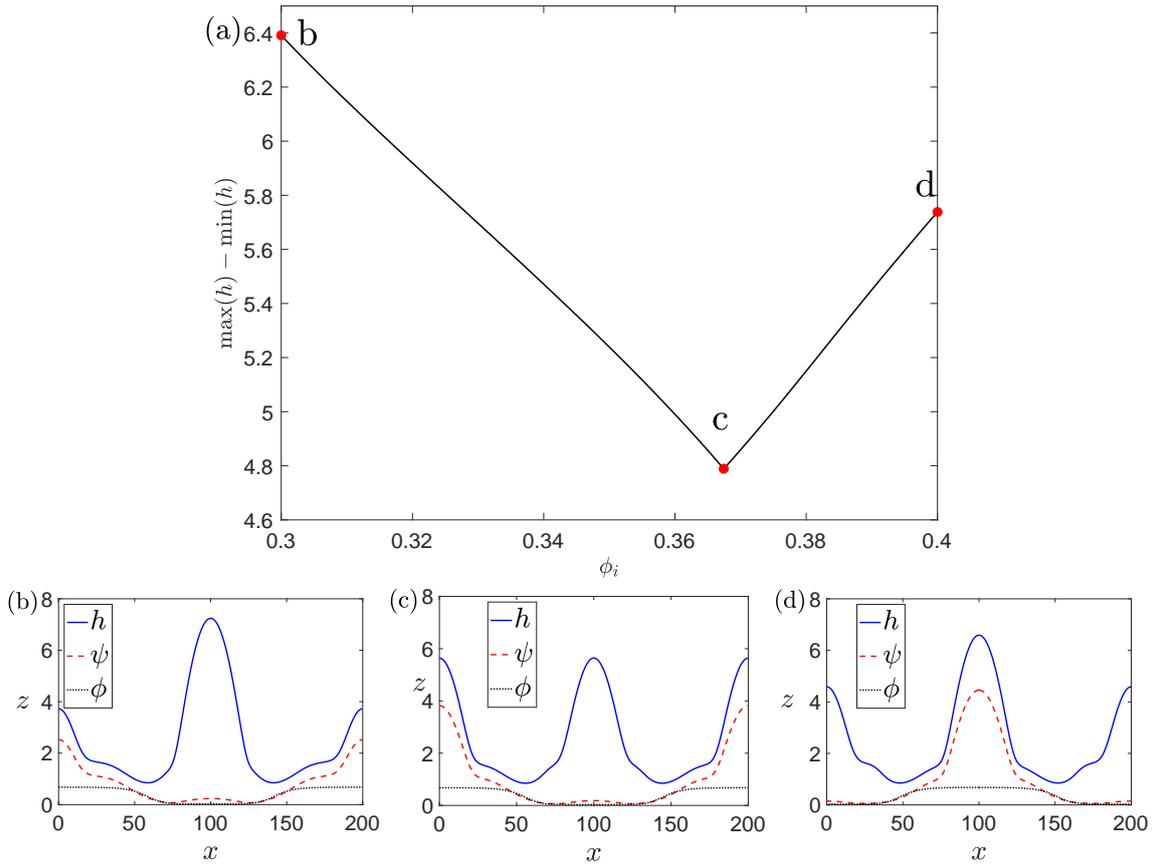
Figure 13: Transition between anti-phase to in-phase at  $L_x = 200$ . (a) Turning point in the maximum difference in film height. (b)-(d) Profiles for  $L_x = 200$  at  $\phi_i = 0.3$ ,  $\phi_i = 0.4$  and the critical concentration  $\phi_i = 0.367$ , with other parameters as in Fig. 11.
