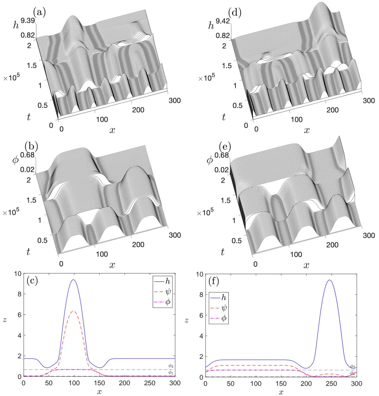
Figure 7: Waterfall plots (using linear  $t$ ) of (a) the film height, and (b) the local colloid concentration, for  $A' = 1$ ,  $K' = 11$ ,  $\alpha' = \beta' = 100$ ,  $\epsilon' = 4000$ ,  $a^2 = 100$ ,  $h_i = 2.5$  and  $\phi_i = 0.4$ . Panel (c) displays the final equilibrium profiles. Panels (d)–(f) show similar results, but with  $\phi_i = 0.3$ , corresponding to a decrease in the total amount of colloids in the system.
