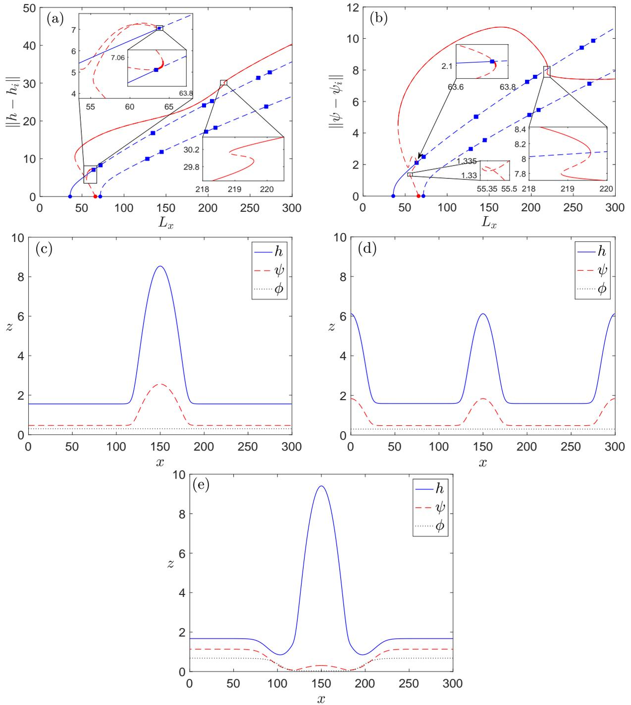
Figure 11: (a)–(b) Bifurcation diagram for parameters as in Figs. 7(d)–(f), where now a second blue line corresponding to a double-droplet profile is depicted. The solid lines correspond to stable solutions, whereas the dashed lines correspond to unstable solutions. (c)–(e) Equilibrium profiles from the film height mode (c) first film height branch and (d) second film height branch; (e) equilibrium profiles from the colloid film mode.
