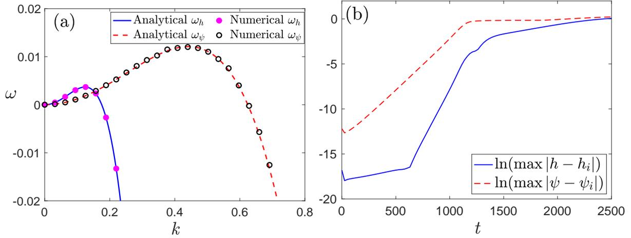
Figure 6: Results for a case with  $A' = 1$ ,  $K' = 0.13$ ,  $\alpha' = 1$ ,  $\epsilon' = 0.5$ ,  $a^2 = 10$ ,  $h_i = 2.5$  and  $\phi_i = 0.4$ . (a) Dispersion relation calculated numerically via Eqs. (51) and (52) using  $\epsilon_h = 10^{-7}$ ,  $\epsilon_\psi = 10^{-5}$  (symbols) compared to the analytic results in Eqs. (33) and (34) (lines). (b) Measure of the evolution [c.f. Eq. (53)].
