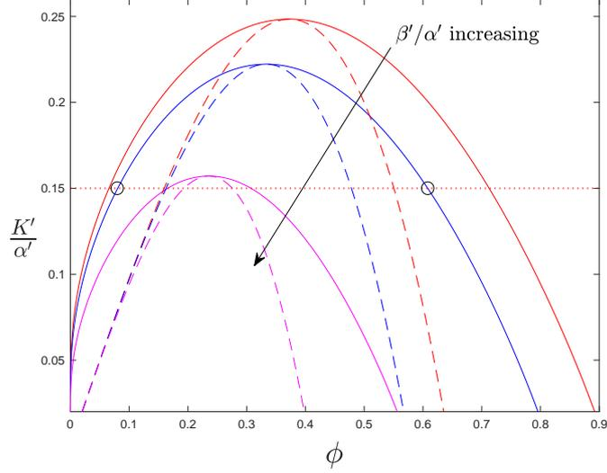
Figure 2: Bulk colloid phase diagram in the plane of dimensionless temperature  $K'/\alpha' = k_B T / (\alpha a^3)$  versus colloid concentration  $\phi$ , for the three values of  $\beta'/\alpha' = \beta/\alpha = 0.8, 1$  and  $2$ . The solid lines are the binodals and the dashed lines are the corresponding spinodals. The circles identify coexisting colloid concentrations for the particular temperature  $K'/\alpha' = 0.15$  and  $\beta'/\alpha' = 1$ , that are referred to in § 4.1.
