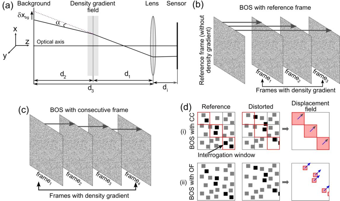
**Fig. 1:** BOS theory. (a) A simple schematic of the BOS principle, (b) BOS measurement with respect to a reference frame, (c) BOS measurement with consecutive frames, and (d) illustration of measurement of the displacement vectors for two popularly reported reconstruction techniques: cross correlation-BOS and optical flow-BOS.
