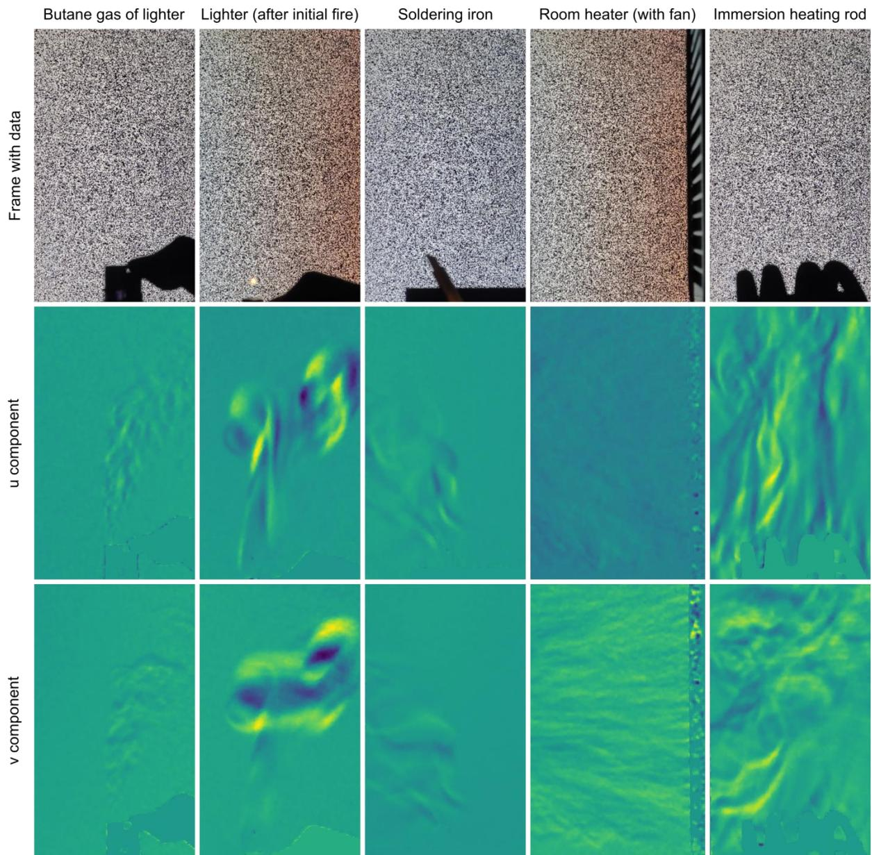
**Supp. Fig. 5:** u- and v-components of the net displacement field reconstructed using the pocket schlieren for the five different schlieren objects- butane gas of lighter, lighter flame, soldering iron, room heater and immersion heating rod, respectively.
