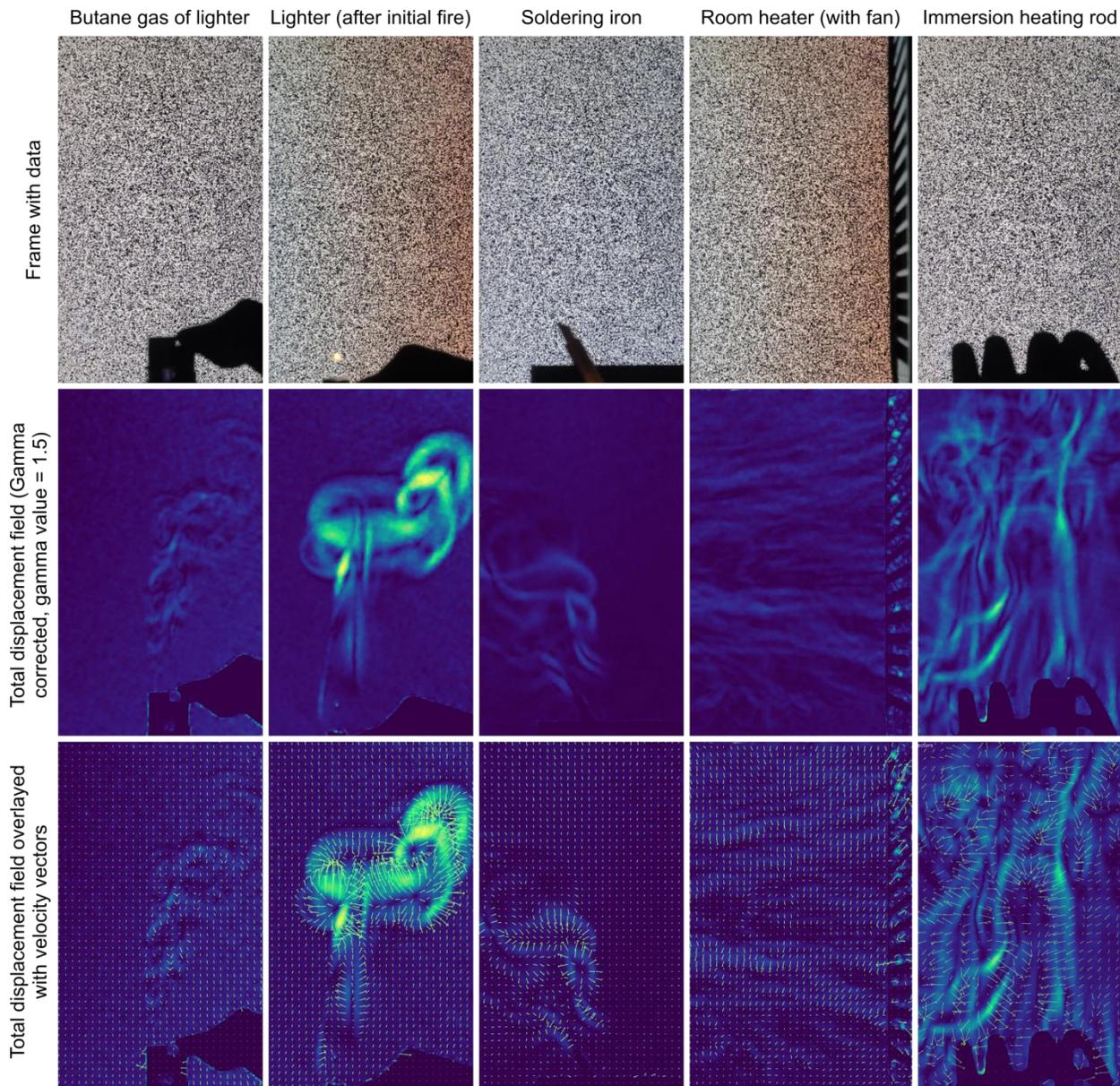
**Fig. 5:** Pocket Schlieren assisted calculation of displacement field and velocity vectors inside flow. Left to right: Different samples used for creating flow which include butane gas lighter, lit lighter, soldering iron, room heater, and immersion heating rod. Top to bottom: a reference data frame, displacement field, and velocity vectors overlaid on top of the displacement field.
