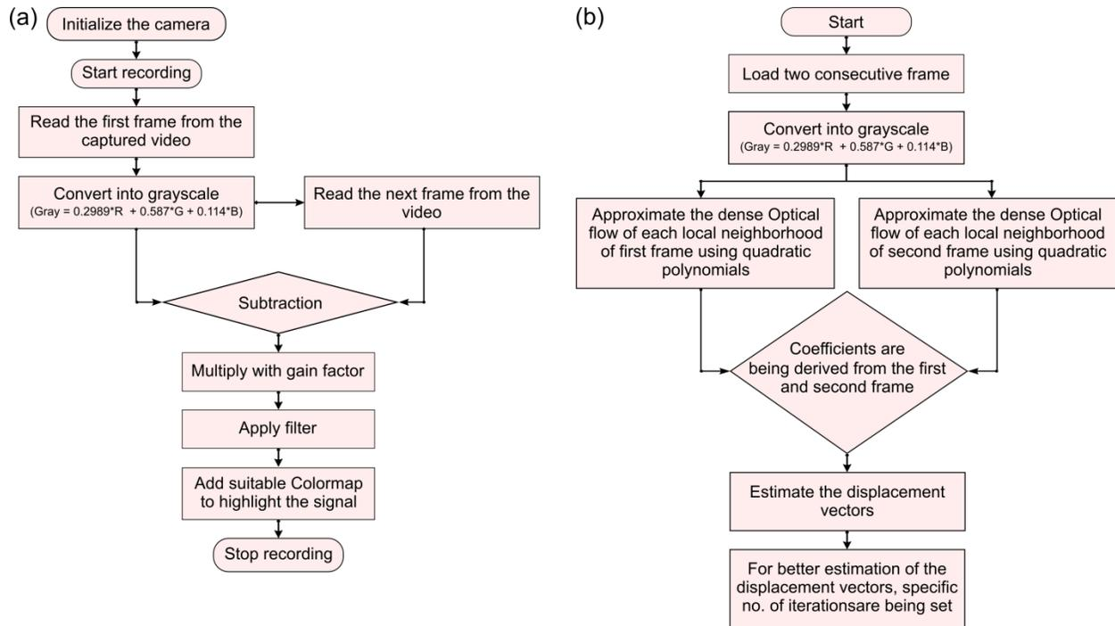
**Supp. Fig. 3:** Pocket schlieren app algorithms. (a) The workflow of the CFS technique, and (b) the Gunnar Farneback algorithm.
