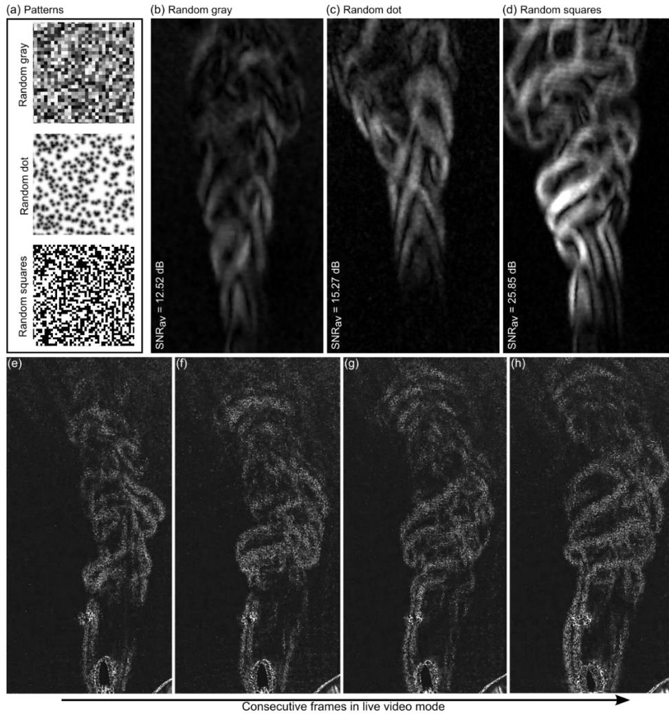
**Fig. 3:** Optimization of the patterned background for Pocket Schlieren. (a) Three patterns under consideration: random gray, random dot, and random squares, respectively, (b)-(d) The reconstructed OF-based BOS results for each of the backgrounds. The noted SNRs are average from eight results, (e)-(h) four consecutive frames recorded using CFS-based live BOS mode. Live BOS performed at 45-50 FPS in 720p resolution. The brightness of the images is enhanced for better visualization.
