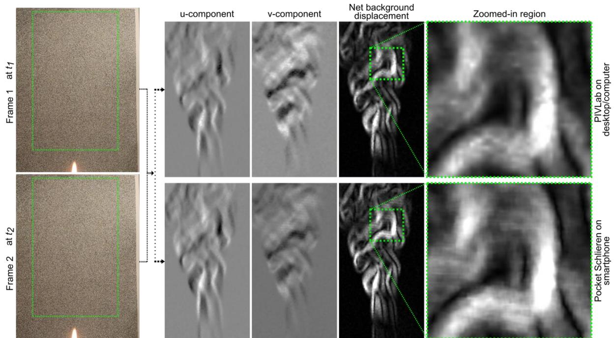
**Fig. 4:** Qualitative comparison of the results obtained from PIVLab and our OF-based Pocket Schlieren app.
